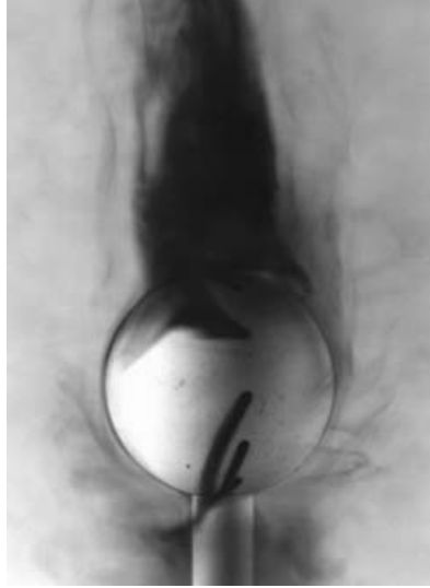
FIGURE 1. Upstream separation on a sphere. Flow is from top to bottom. Image from unpublished flow visualization by Joubert and Wang.
